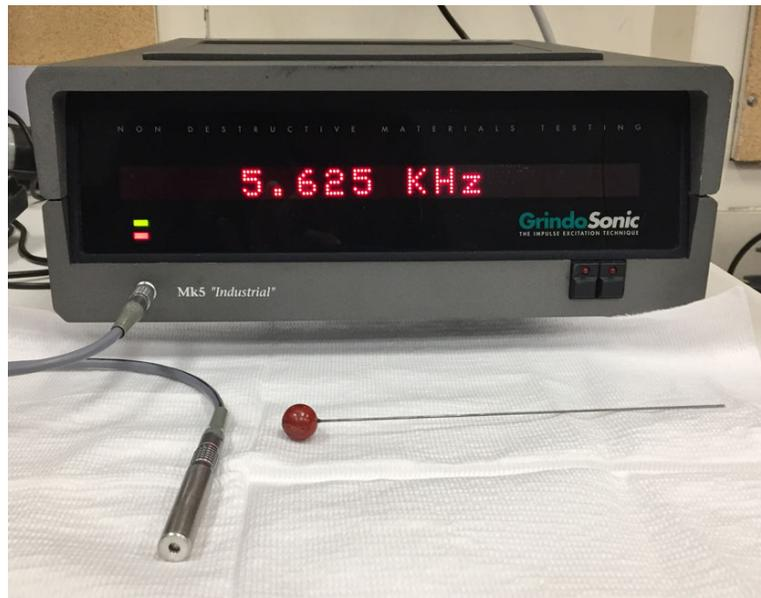
Figure 9. GrindoSonic Mk5 fundamental frequency modulus system.
